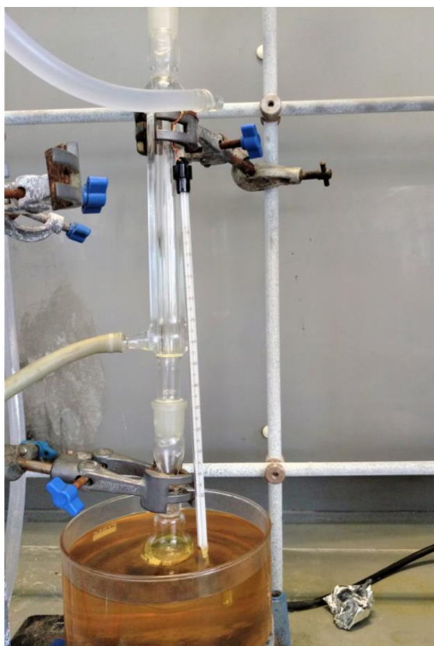
Figure 3.5; Batch transesterification reaction of Jatropha curcas and waste cooking oils.
