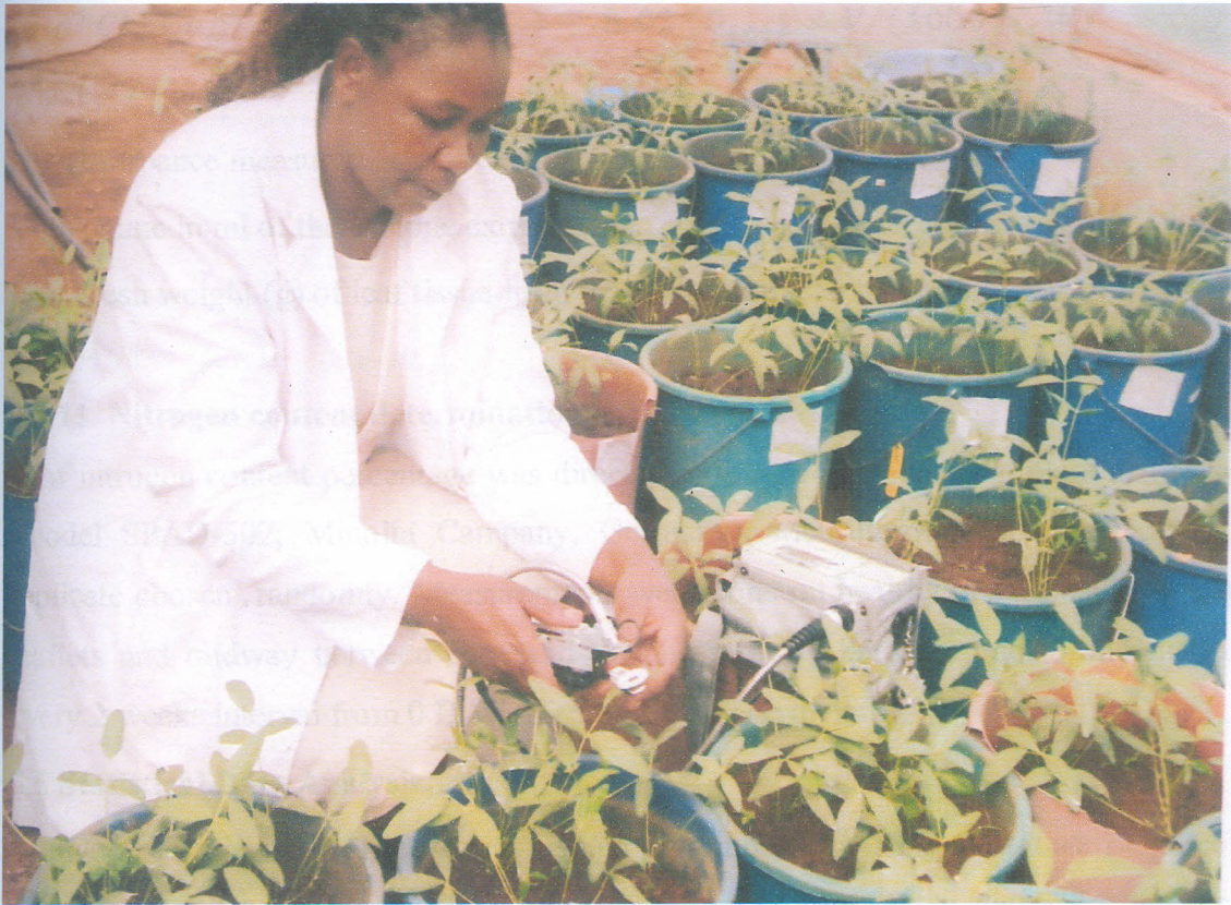
Plate 1: Demonstration of chlorophyll fluorescence measurements using a portable fluorescent monitoring system on five week old Bambara groundnuts.
