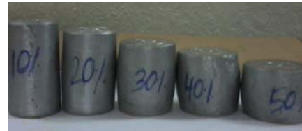
Fig.2.(e): Al-10Si-8%TiB 2 composite specimens showing bulge profiles at various deformation stages under compression testing at aspect ratio 1.5.
