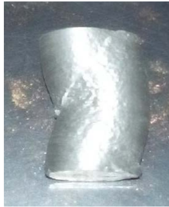
Figure.14 Compressive test specimen Sample 1 - (Aluminium 97%, E-glass fiber 3%)
