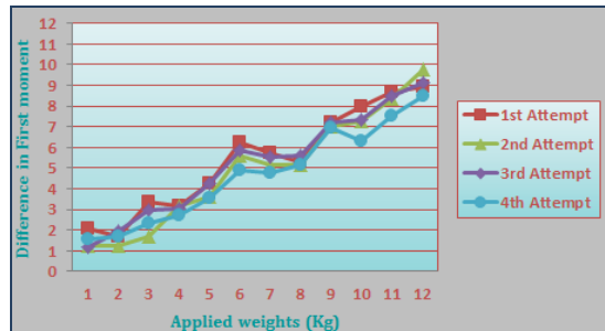
Figure (7): Difference in first moment against the applied weight with five ridges of 3mm diameter
