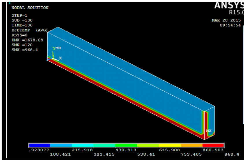
Figure 5.7: Nodal Solution for the FEM model at 130min.
