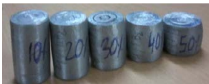
Fig.2.(d): Al-10Si-6%TiB 2 composite specimens showing bulge profiles at various deformation stages under compression testing at aspect ratio 1.5.
