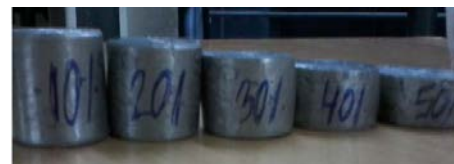
Fig.1(c): Al-10Si-4%TiB 2 composite specimens showing bulge profiles at various deformation stages under compression testing at aspect ratio 1.0.
