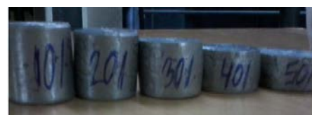
Fig.1(d): Al-10Si-6%TiB 2 composite specimens showing bulge profiles at various deformation stages under compression testing at aspect ratio 1.0.
