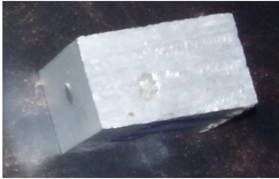
Figure.19 Hardness test specimen Sample 1 - (Aluminium 97%, E-glass fibre 3%)
