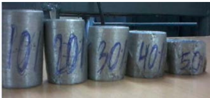
Fig.2.(b): Al-10Si-2%TiB 2 composite alloy specimens showing bulge profiles at various deformation stages under compression testing at aspect ratio 1.5.
