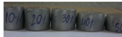
Fig.1(a): Al-10Si alloy specimens showing bulge profiles at various deformation stages under compression testing at aspect ratio 1.0.
