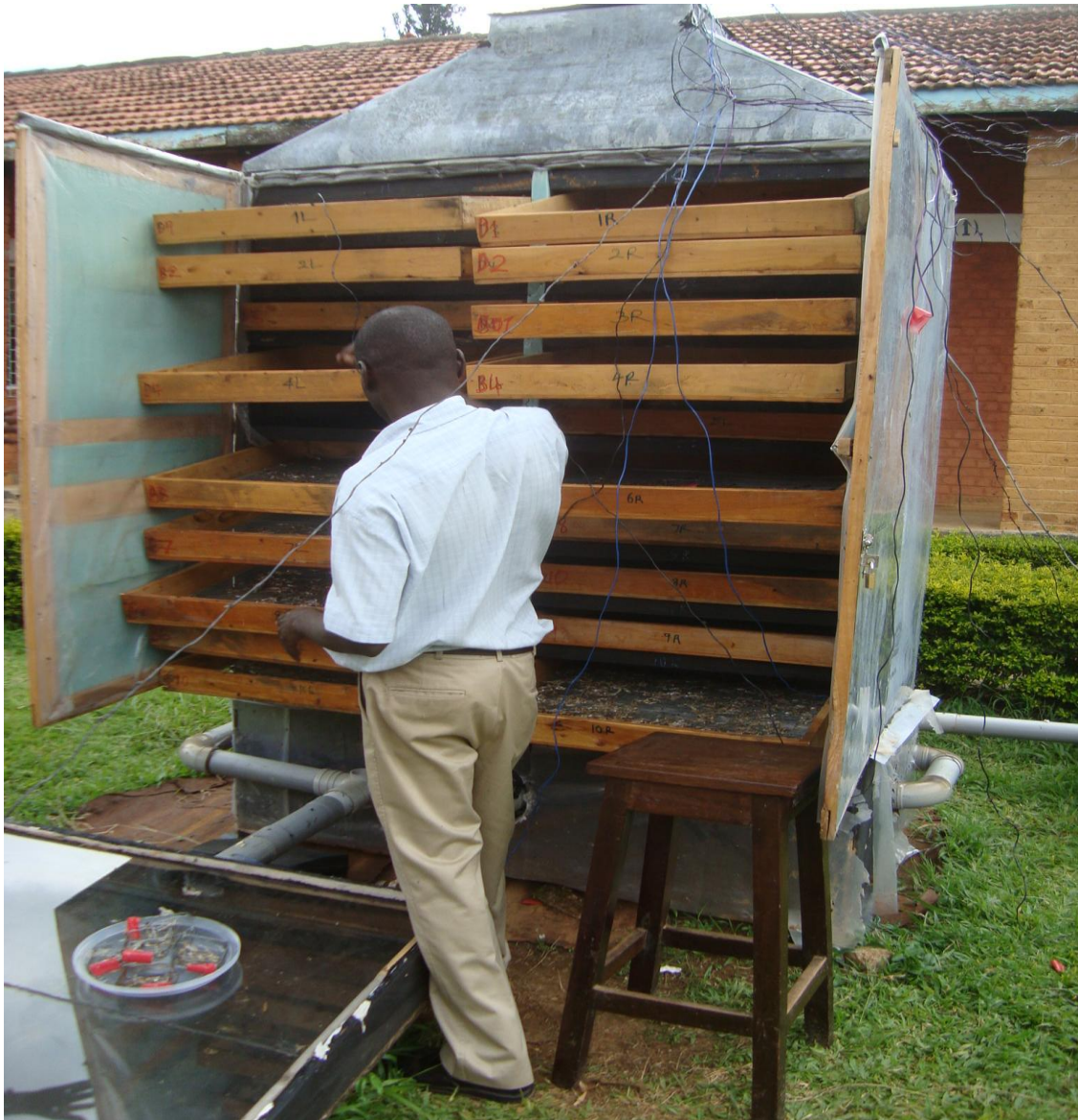
Figure 3.3: Pictorial view of the indirect cabinet solar dryer loaded with R. argentea fish
