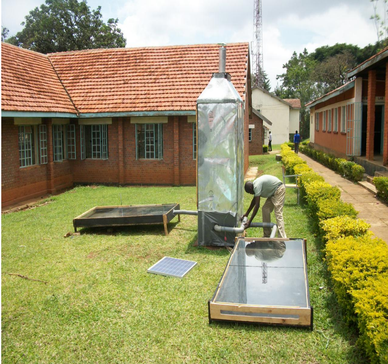
Figure 3.2: Pictorial view of the prototype indirect cabinet forced convection solar dryer, developed at Maseno University, Kenya.
