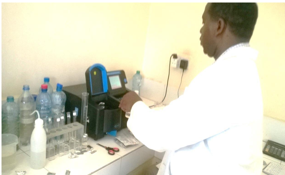
Plate 3.9: Phosphate, nitrate and COD estimation using a spectrophotometer (photograph taken on 6.5.15 by A. Mbeke).
