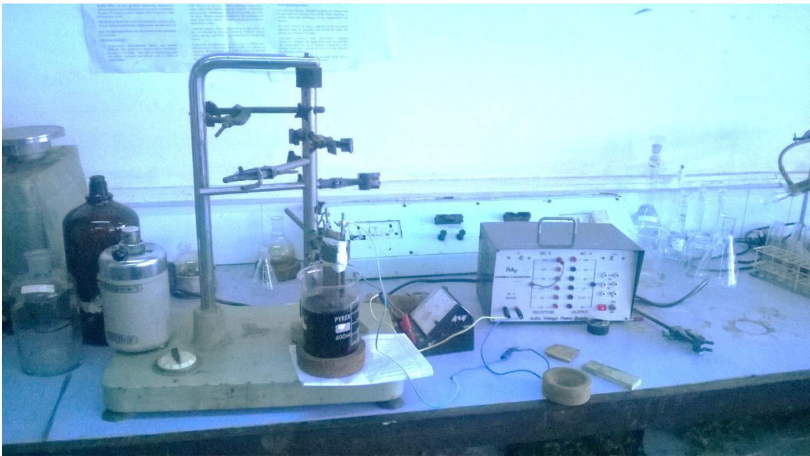
Plate 3.7: Electrocoagulation experimental method in progress. (photograph taken on 6.5.15 by A. Mbeke
