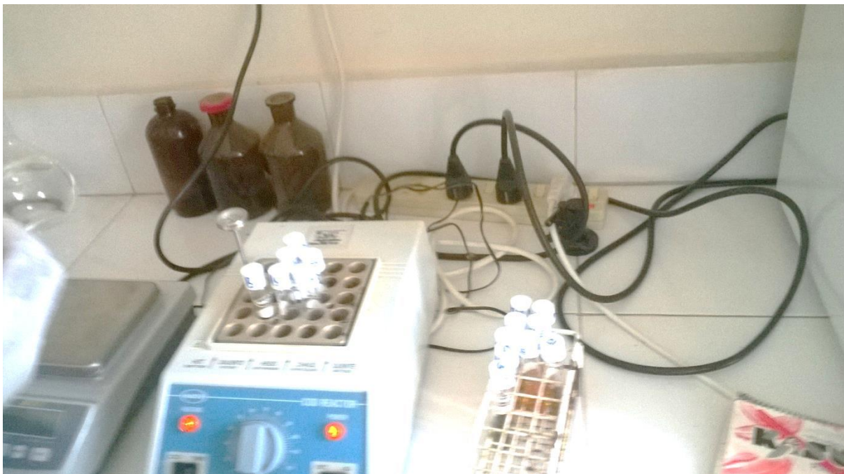
Plate 3.6: Waste water samples incubated in a COD reactor for two hours and the BOD trak bottles (photograph taken on 18.6.2015; by A. Mbeke).
