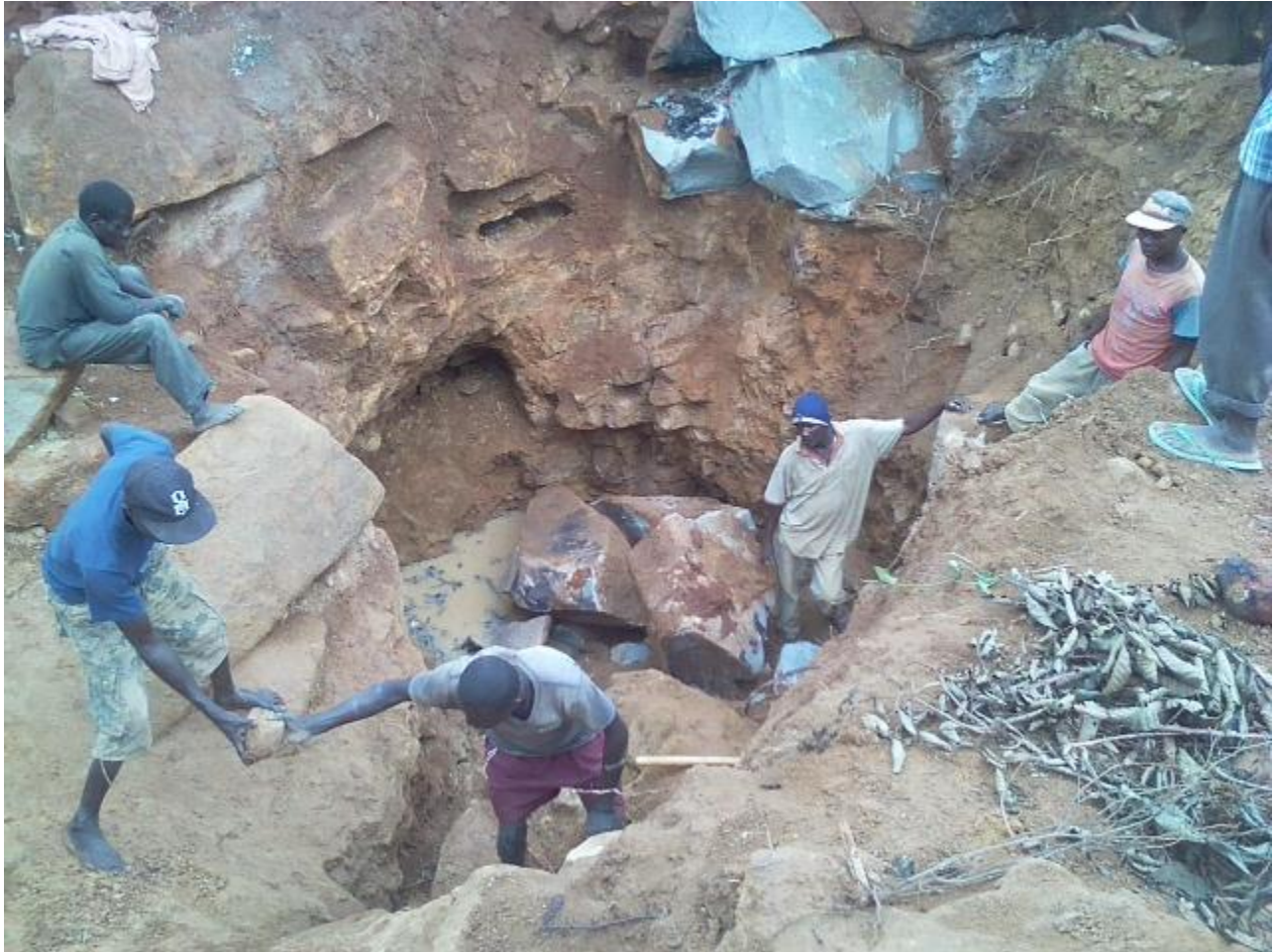
Plate 4.4: Artisanal gold miners removing rock debris from a gold pit in Karemo division
